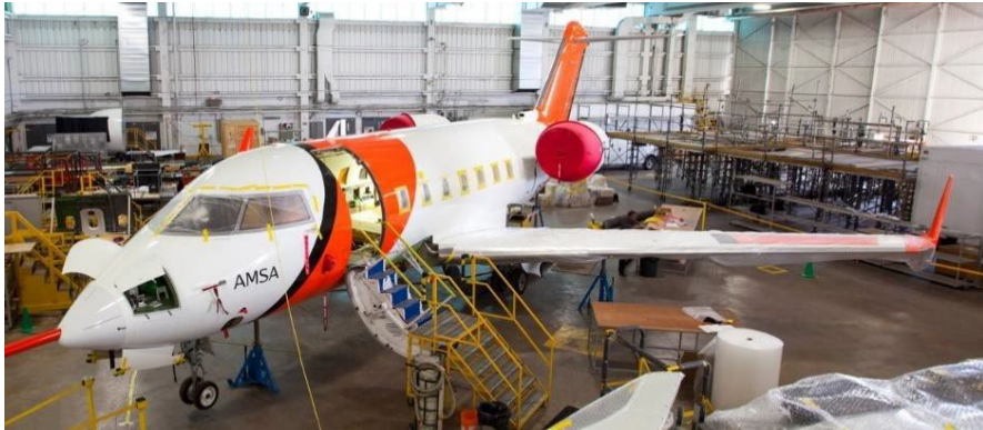
Bombardier CRJ regional jet undergoing maintenance in YYZ hangar
