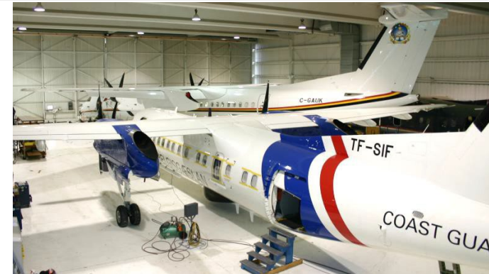
Bombardier Dash 8 being modified for coast guard surveillance
